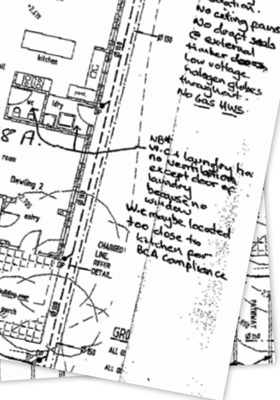
These homes didn't comply with the plans provided through energy ratings software
